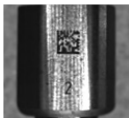
Figure 8: Laser-marked code on a metal cylinder
